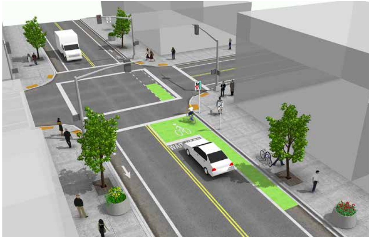
Example of a Bike Box at a Signalized Intersection with a Bike Lane Approach Source: NACTO
