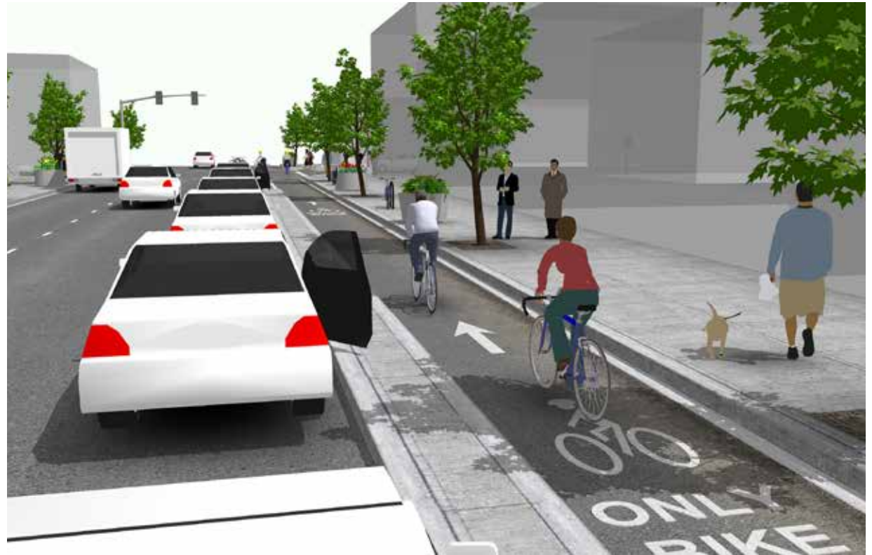
Parking protected bike lanes use a wider buffer to prevent “dooring.” Source: NACTO
