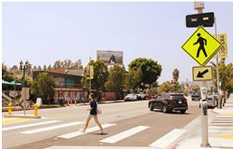
**Crosswalk with Flashing Beacon** such as Rectangular Rapid Flashing Beacons (RRFBs), enhance the visibility of marked crosswalks. Flashing lights and additional signage alert drivers to where they may expect people to be crossing the street.
