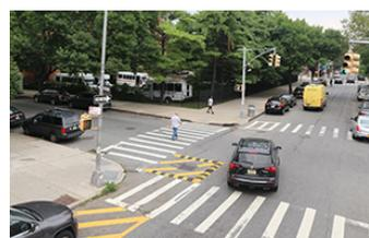
**Left Turn Traffic Calming** reduces the speed of drivers' left turns and reduces the risk of a pedestrian collision.
