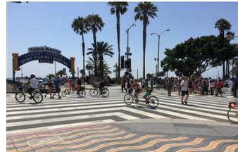
**Scramble Crosswalks** give pedestrians exclusive access to an intersection by stopping vehicular traffic on all approaches, allowing pedestrians to cross diagonally or conventionally.
